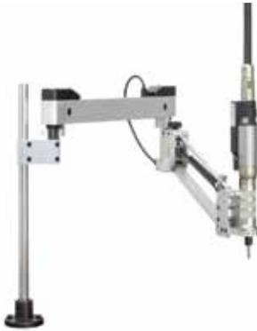
The Tracer Arm for the EH2 vastly improves operating efficiency and ensures error-proof assemblies. It is equipped to detect the position of the EH2 tool and compare it to preprogrammed position data. The operator must perform the fastening sequence properly or the tool is disabled. Fastening data is stored and can be exported for qualification and analysis.
